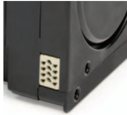
F CINCH connector (female connector mounted on HOPPER)
